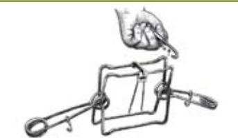
Figure SK4a. Using safety gripper
